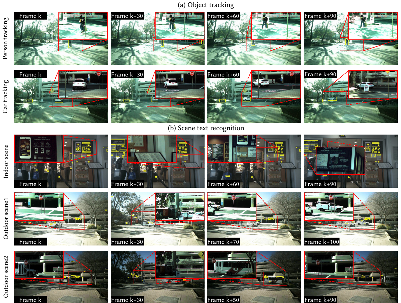
Fig. 6. Policy-based foveated imaging in real-world captures. Under realistic bandwidth and acquisition latency constraints, our proposed method runs in real time on our 200 MP-resolution foveated imaging prototype. We demonstrate expected smooth-pursuit scanpaths for (a) object tracking and saccading scanpaths for (b) scene text recognition across diverse scenes and lighting conditions.
